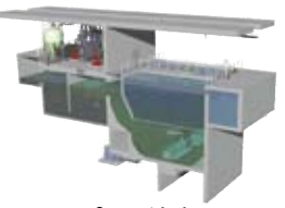
ACTIFLO® provided needed capacity without the large surface area requirements.
