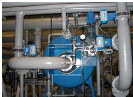
Auto-Jet® Pressure Leaf Filters are designed to remove fine clays down to 0.5-1.0 micron size.
